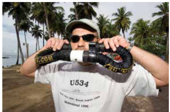
Figure 6. Loop check. Richie Kohler checks the non-return valves in his loop. Photo courtesy Jill Heinerth.
