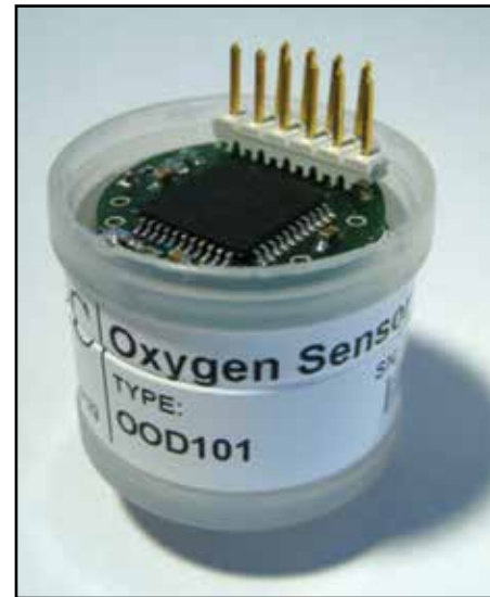
Figure 5. Prototype of our "smart" galvanic O 2 sensor.
