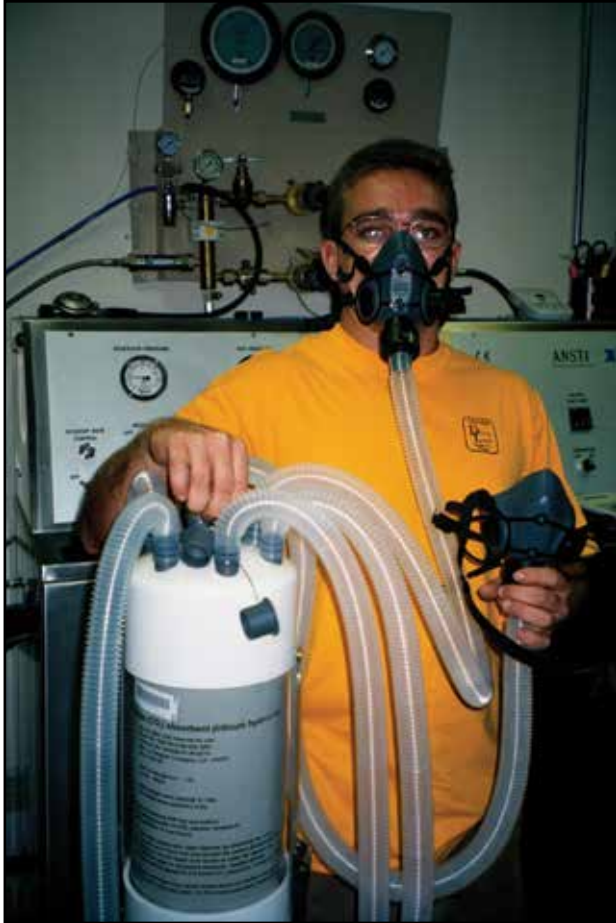
Dive Lab six-man CO 2 scrubber for submarine rescue use. Photo courtesy Dive Lab.
