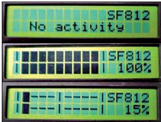
Figure 12. Photograph of the diver's display during different phases of a dive. The "SF812" refers to the absorbent used when the photo was taken.
