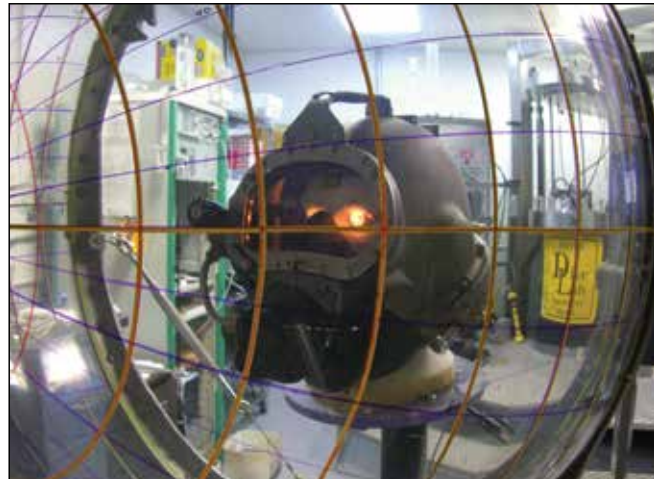
Figure 3. Field-of-vision test on a helmet. Photo courtesy Dive Lab.
