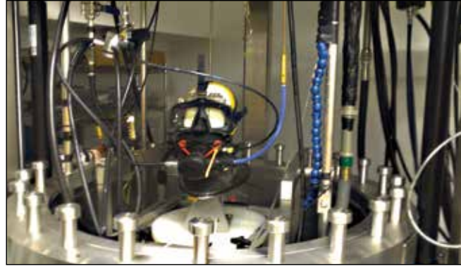
Figure 2a. Open-circuit band mask in ANSTI test chamber. Photo courtesy Dive Lab.
