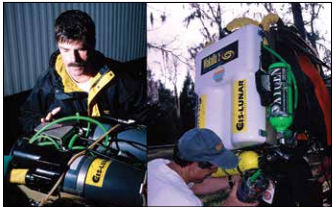
Figure 21. Final kitting up with the dual backmounted rebreather, January 1999. The small green tank is offboard oxygen; the small yellow tank is drysuit inflation argon supply. A second oxygen tank was placed inside the shell between the two CO 2 canisters.
