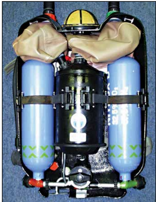
Figure 6. Photo of the Dräger FGT 1/D semiclosed-circuit rebreather. Photo by John R. Clarke.
