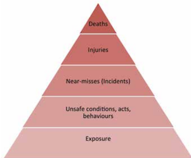
Figure 1. The accident pyramid (Heinrich, 1936), modified by the author (accidents = injuries and deaths).
