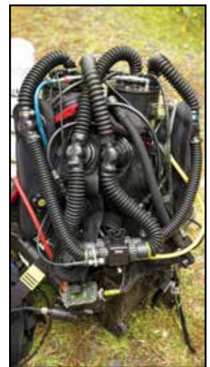
Figure 5. For deep dives in the Pearse Resurgence, Craig Challen uses a Twin Megalodon rebreather, with the two loops accessible by a custom-made dual bailout valve. This allows the diver to change from one loop to another with the flick of a switch. Photo by Richard Harris.
