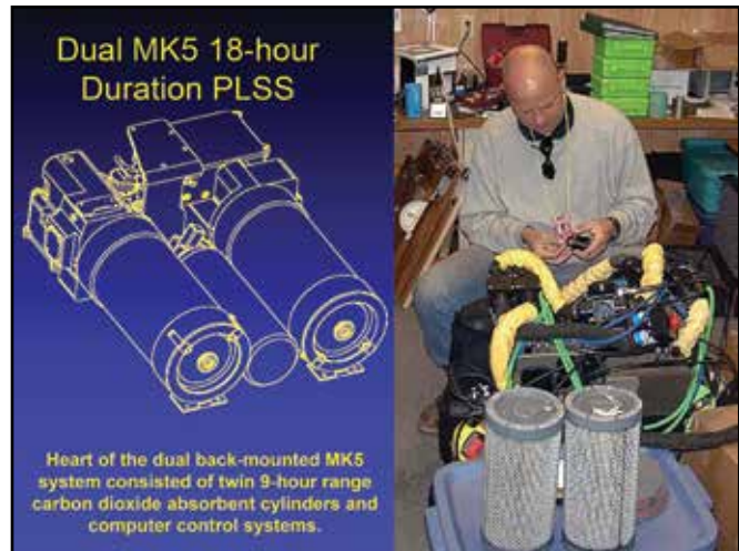
Figure 20. Assembly of the dual backmounted rebreather. The device used two radial hydrophobic carbon-dioxide absorbent canisters.
