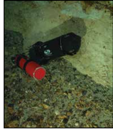
Figure 4. Bailout and a CCR are staged along the cave line. In case of light failure, divers can navigate out and find extra equipment placed for contingencies. Photo by Pete Nawrocky.
