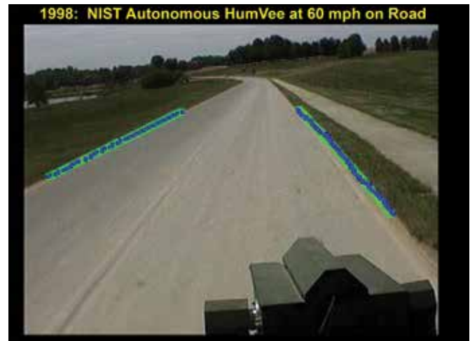
Figure 34. An illustration of machine vision serving as the “eyes” for an intelligent system (in this case, an unmanned ground vehicle).
