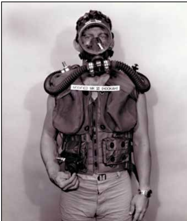
Figure 4. Photo of the U.S. Navy MK VI semiclosed-circuit rebreather. U.S. Navy photo.
