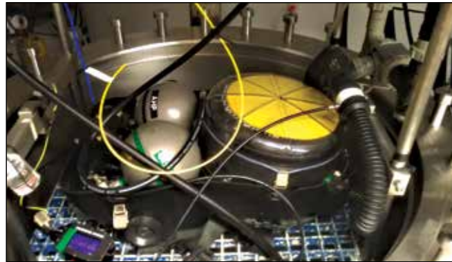
Figure 2b. Mk 16 closed-circuit rebreather in ANSTI test chamber. Photo courtesy Dive Lab.
