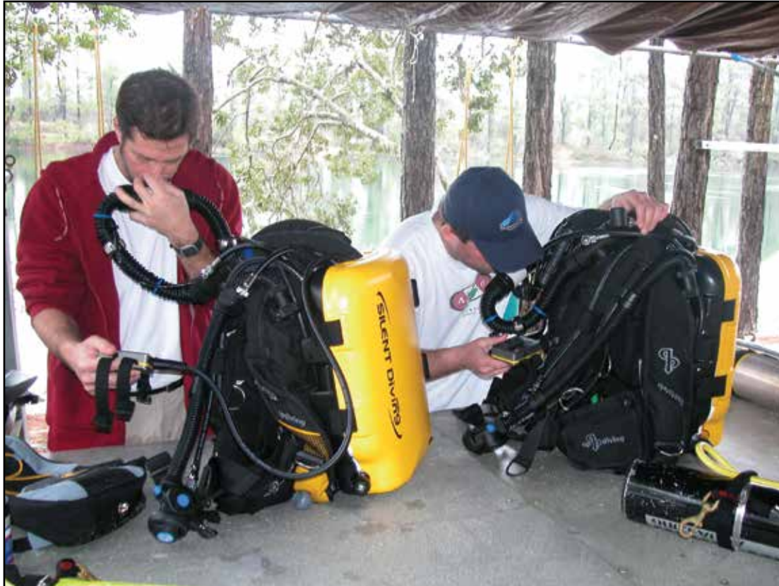
Prebreathing your CCR before donning is paramount to confirm the unit is assembled and functioning correctly prior to entering the water. Photo courtesy Richie Kohler.
