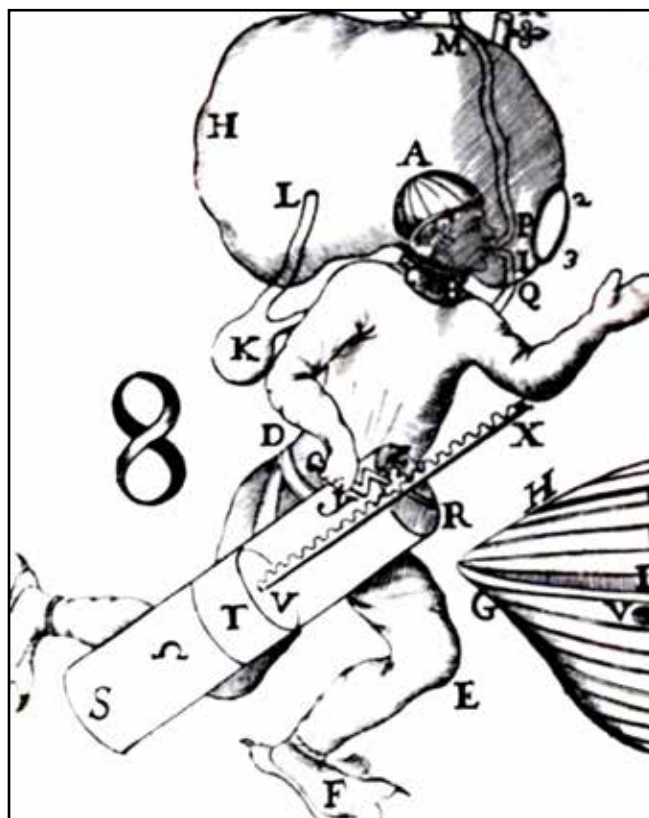
Figure 1. One of the earliest "rebreather" designs. In 1680 Giovanni Borelli envisioned a diver carrying a large bag of air from which the diver breathed, as necessary. Image courtesy of Cayman Island Twilight Zone 2007 Exploration, Giovanni Borelli 1680, Library of Congress, July 1, 1909, NOAA-OE.
