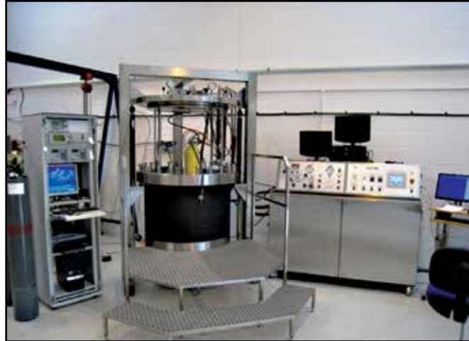
Figure 1. The ANSTI Life-Support Equipment Test Facility set up for measurement of breathing mechanics, scrubber capacity, and oxygen control in open- and closed-circuit breathing apparatus to a depth of 200 msw (656 fsw).
