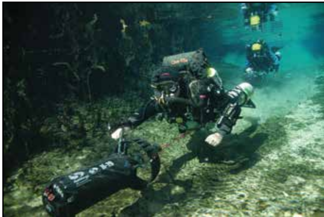
Figure 1. CCR cave divers utilize DPV units to extend exploration. Appropriate gas planning, including staging bailout bottles, is critical for proper exiting in case of DPV or CCR failure. Photo by Pete Nawrocky.
