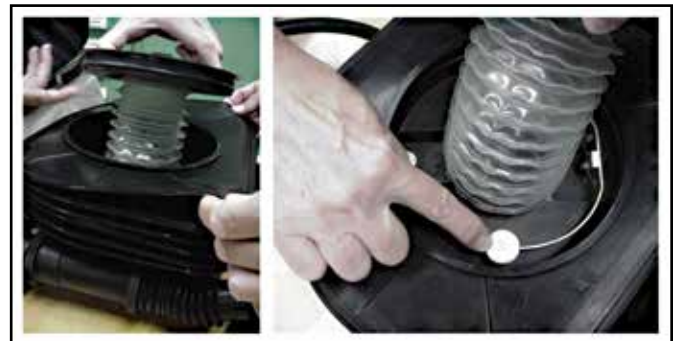
Figure 27. Oxymix 3C inner (exhaust) and outer bellows (left and right panel). The demand valve actuator is pointed out in the right panel. U.S. Navy photo.
