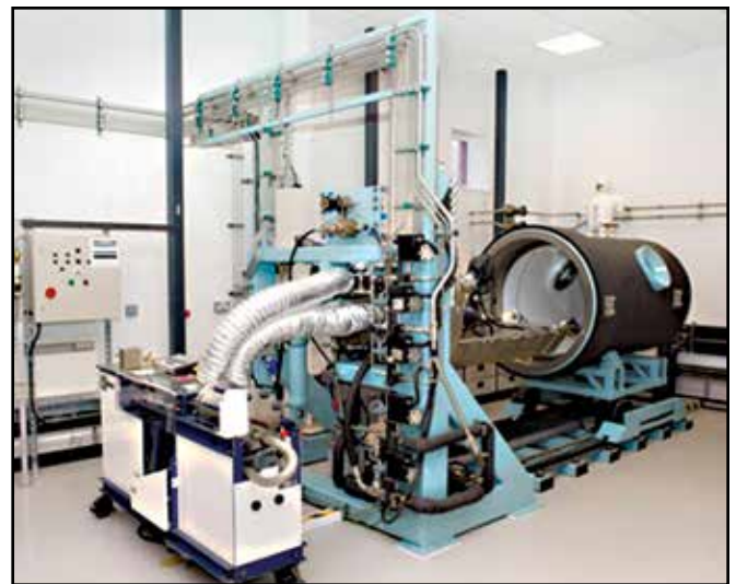
Figure 1. Unmanned test chamber and breathing simulator.
