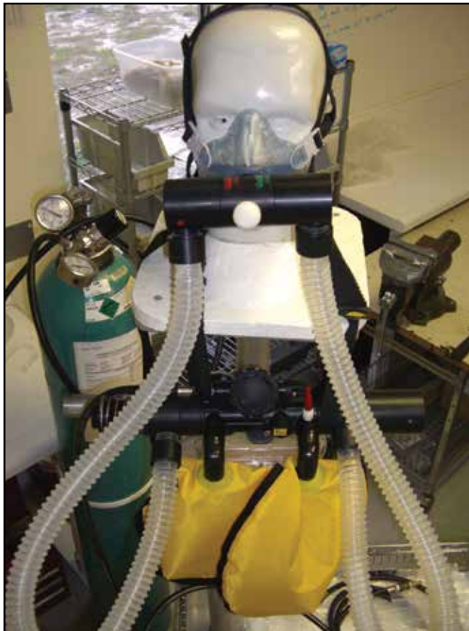
Dive Lab oxygen rebreather for submarine rescue use. Photo courtesy Dive Lab.
