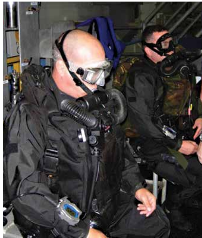
Figure 14. Divex Shadow Excursion diver instrumented with an oxygen sensor and data recorder. Photo by John R. Clarke.
