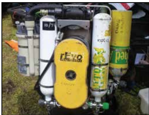
Figure 4. A close up of Sandy's twin unit, the "R2D2." The extra cylinder on the right-hand side is for drysuit inflation. Photo by Richard Harris.
